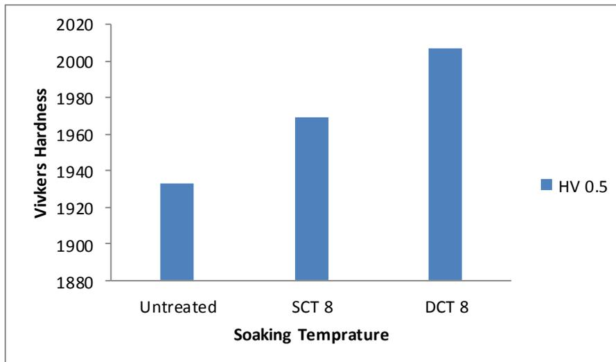
**Figure 4:** Microhardness value of untreated and cryotreated tools
