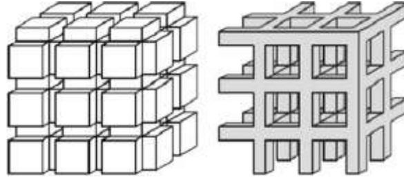
**Figure 1:** Hard tungsten carbide skeleton and soft cobalt binder form a composite of WC-Co [4].
